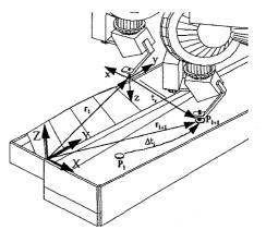
Fig. 2 Relationship between the moving object and gripper
